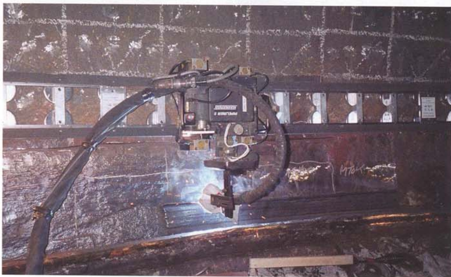
Fig. 5 — The orbital welding equipment is shown on the workpiece, which was preheated to 300°F.
